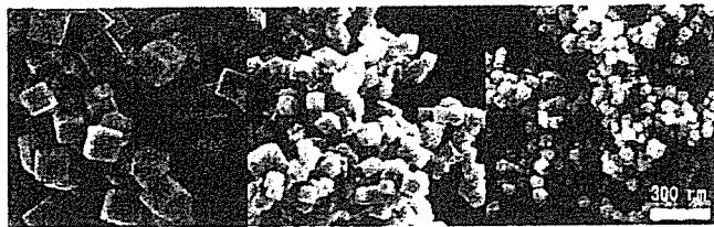
Fig. 6. SEM micrographs of the FeCo alloy nanoparticles (a) \text{Fe}_{73}\text{Co}_{23} , (b) \text{Fe}_{74}\text{Co}_{26} , and (c) \text{Fe}_{57}\text{Co}_{43} synthesized in EG.
