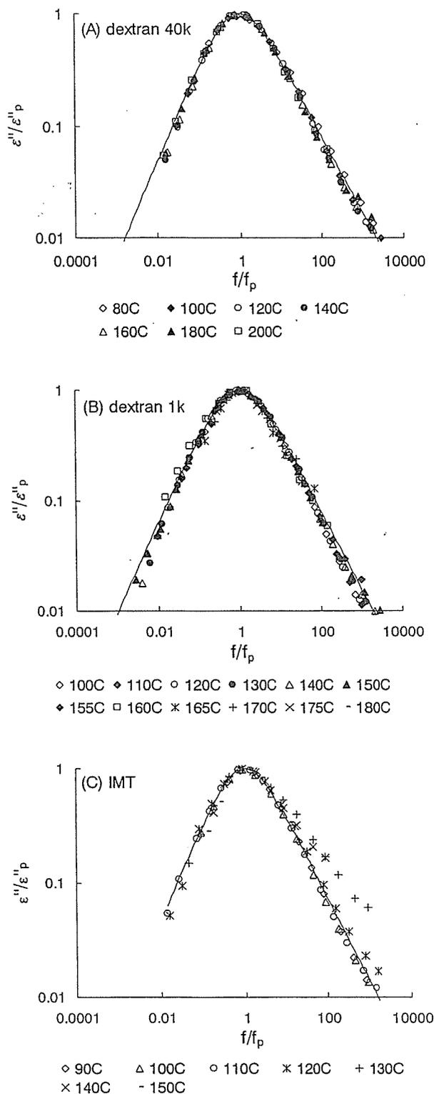
**Figure 5.** Normalized plot of imaginary permittivity for the Maxwell-Wagner-like process observed in freeze-dried dextran 40k (A), dextran 1k (B) and IMT (C) with a Teflon sheet inserted.
