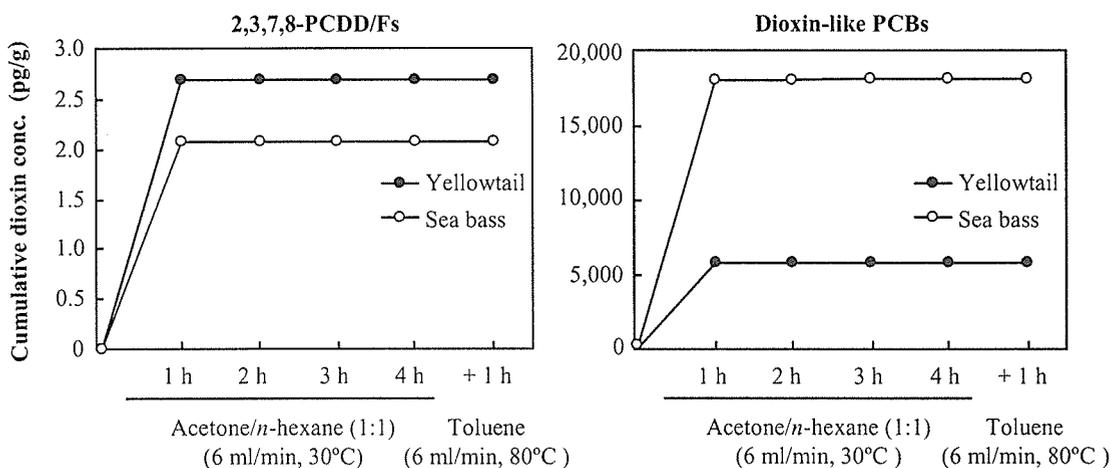
**Figure 2** Dioxin concentrations in the high-speed solvent extraction under various extraction conditions. Two popular fish samples were serially extracted by the high-speed solvent extraction with acetone/*n*-hexane for up to 4 h under 30°C and then extracted with toluene for 1 h under 80°C. The hourly extracts were spiked with <sup>13</sup>C<sub>12</sub>-labelled internal standards and cleaned up for HRGC/HRMS analysis.
