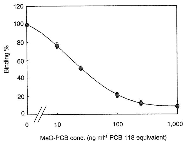
Fig. 2. Standard curve for the ELISA. Circles represent the mean binding from six separate assays performed on different days. Bars represent SDs. The y-axis shows the percentage of binding:  $\text{Binding \%} = A^+/A^- \times 100$ . Here,  $A^+$  is the absorbance in the presence of standard and  $A^-$  is the absorbance in its absence.
