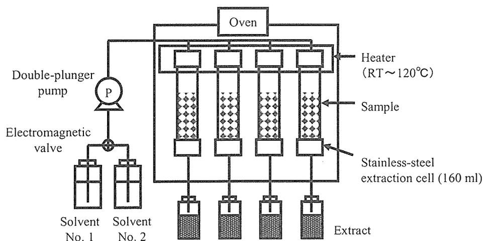
**Figure 1** Schematic diagram of the extractor (SE-100)
