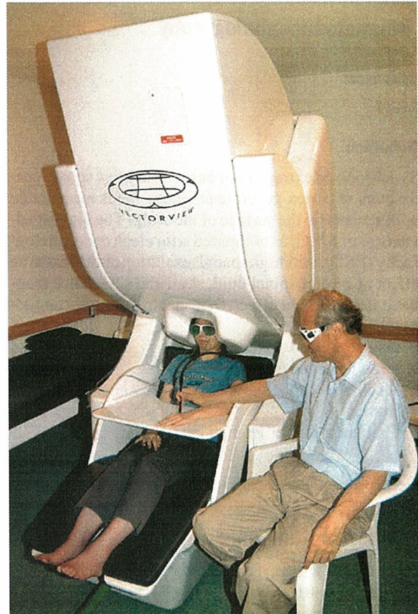
Magnetoencephalography in Assessment of Pain in Humans, Figure 1 The procedure using our MEG device (VectorView 306-channels, Elekta Neuromag Oy, Helsinki). The laser stimulator is set outside the shielded room because of its large magnetic artifacts and the laser beam is applied to the subject's hand through optical fibers. The laser beam can be applied any part of the body except the eyes, so both the experimenter and the subject must wear special glasses or swimming goggles.
