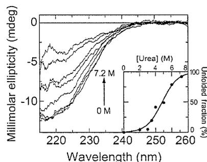
Fig. 2. Effect of urea on hDAAO conformation. CD spectra were recorded after the addition of increasing urea concentration (0–7.2 M); each spectrum was determined on individual sample prepared by mixing appropriate volumes of protein (0.1 mg protein/ml), 8 M urea in buffer, and plain buffer (50 mM sodium pyrophosphate, pH 8.3), at 15 °C. Inset: equilibrium denaturation curve from the CD signal at 220 nm.
