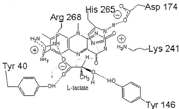
Fig. 5. Schematic representation of the reaction mechanism on the FMN by the residues Y40, Y146, D174, H265, and R268.
