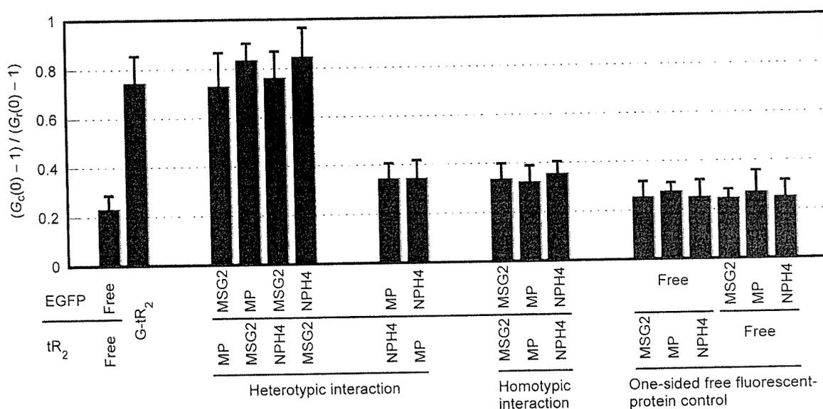
**Fig. 3** Cross ratio  $[(G_c(0)-1)/(G_r(0)-1)]$  determined with FCCS, which corresponds to the fraction of the associated molecules ( $N_c/N_B$ ). MSG2 and MP- and NPH4-CTDs were fused with EGFP or tR<sub>2</sub>. Values shown are the mean and SD of 4–9 measurements.
