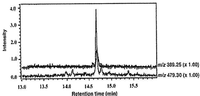
Fig. 1. Detection of leukotriene B<sub>4</sub> as pentafluorobenzyl ester di-trimethylsilyl ether derivative in human urine by gas chromatography-mass spectrometry-selected ion monitoring.
