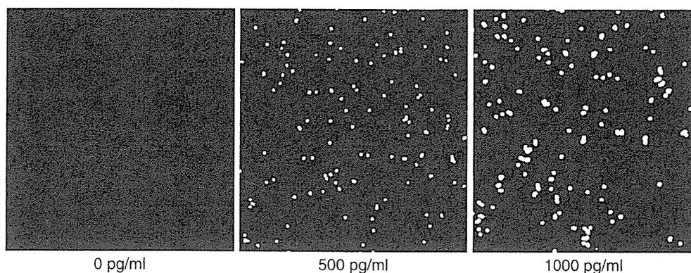
**Fig. 2** Detection of fluorescence-linked beads in the wells with various concentrations of hIFN- $\gamma$ . The intensity of the bead-bound fluorescence increased according to the hIFN- $\gamma$  concentration.
