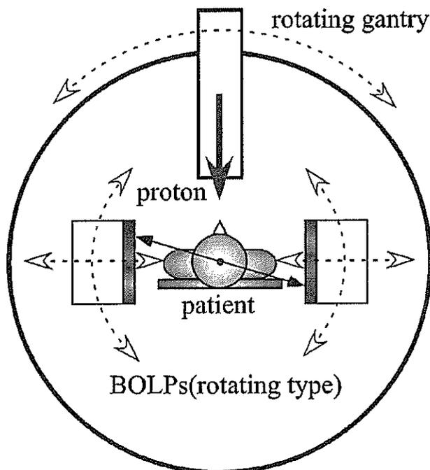
FIG. 10. View of the BOLPs equipped to rotate with the rotating gantry.
