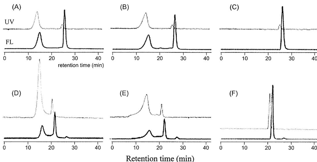
**Figure 2.** GFLC chromatograms of dextran-based CL probes. Samples: (A), 1.0 mg/mL Dex2000-(Lu)<sub>2627</sub>-(Bi)<sub>385</sub>; (B), 1.0 mg/mL Dex50-(Lu)<sub>559</sub>-(Bi)<sub>34</sub>; (C), 0.011 mg/mL Lu; (D), 1.0 mg/mL Dex2000-(ILu)<sub>3262</sub>-(Bi)<sub>275</sub>; (E), 1.0 mg/mL Dex500-(ILu)<sub>321</sub>-(Bi)<sub>15</sub>; (F), 0.011 mg/mL ILu. Injection volume: 10  $\mu$ L. For other chromatographic conditions, see in Materials and Methods.
