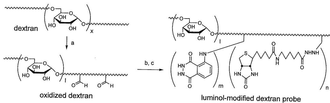
**Scheme 1.** Synthetic route to dextran-based CL probes. Reaction conditions: a,  $\text{NaIO}_4$ , water, room temperature; b, 6-hydrazidohexyl *D*-biotinamide in DMSO then acetic acid, luminal,  $60^\circ\text{C}$ ; c,  $\text{NaBH}_4$  in ethylene glycol,  $4^\circ\text{C}$ .
