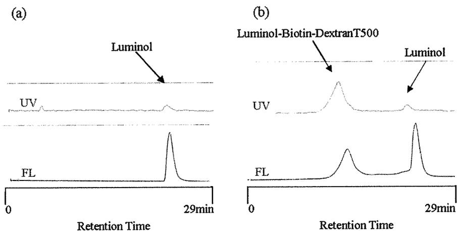
**Figure 3.** GFLC of Luminol-Biotin-DextranT500 polymeric CL compound. Samples: (a) 0.011 mg / mL luminol at 25 min; (b) 1.0 mg/mL Luminol-Biotin-DextranT500 [(Lu)<sub>559</sub>-(Biotin)<sub>34</sub>-(Glc)<sub>3086</sub>] at 14 min. GFLC conditions: injection volume, 10  $\mu$ L; column, TSK gel T2000SW; eluent, 0.1 % (v/v) TFA aqueous solution; flow rate, 1.0 mL/min; UV detection,  $\lambda_{\text{abs}}=275$  nm; FL detection, Ex (mercury lamp)/Em (wavelength cut-filter) =254 nm / > 360 nm.
