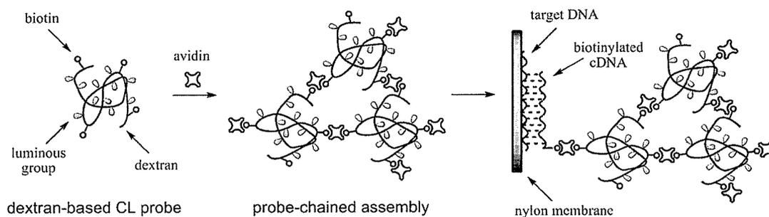
**Figure 1.** Schematic principle for sensitive CL detection of a target DNA by use of luminol- and biotin-containing dextran probe. Conjugation of the dextran-based probe via avidin protein resulted in the formation of a probe-chained assembly. This assembly recognized the biotinylated cDNA that hybridizes with the target DNA.
