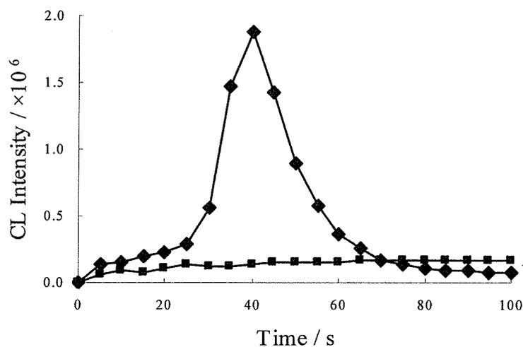
**Figure 5.** CL kinetics of Luminol-Biotin-Dextran T500 compound on nylon membrane. (■) without Fe (III) catalyst, (◆) with Fe (III) catalyst.
