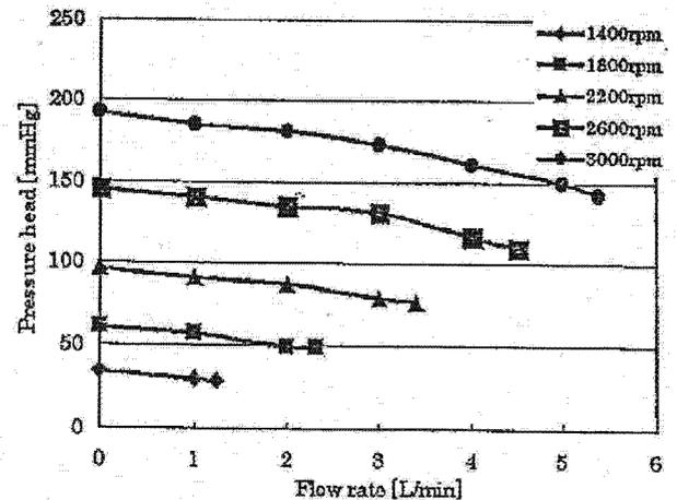
Figure 6. As shown in the graph of pump performance, the CFP generated 5.38 l/min at 3000 rpm when the pump head was 142 mm Hg.
