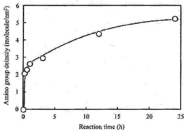
**Figure 2.** Amino group densities on the TiO<sub>2</sub> particle surfaces after modification at 30°C for different reaction times.
