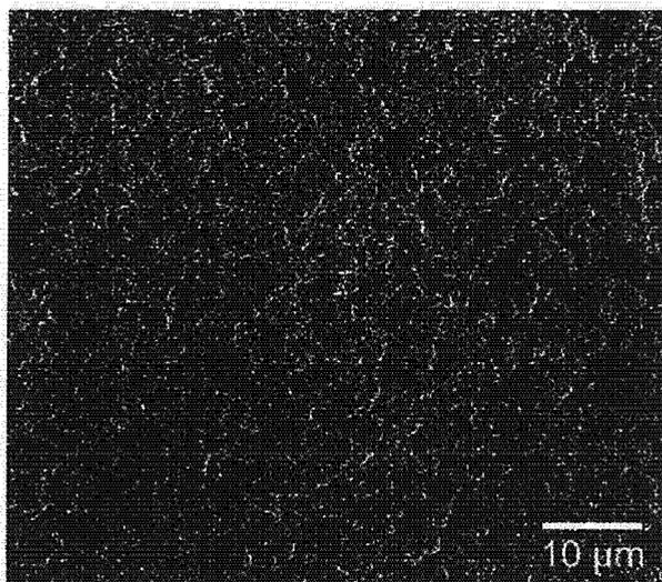
**Figure 1.** A typical SEM photograph of a surface of amino-group-modified TiO<sub>2</sub>/silicone composite sheet, showing a 60% covered surface by the modified TiO<sub>2</sub> particles (amino group density, 3.0 molecules/nm<sup>2</sup>).
