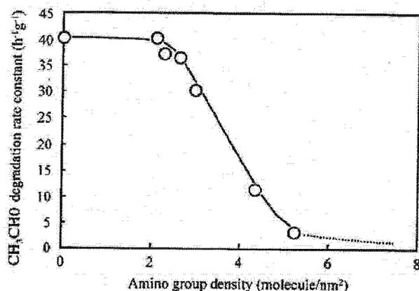
**Figure 3.** Relationship between the amino group density on the TiO<sub>2</sub> particle surfaces and the degradation rate constant calculated from the decrease of CH<sub>3</sub>CHO concentration by UV irradiation (>300 nm; 2000 μW/cm<sup>2</sup>; 2 h).
