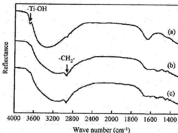
**Figure 4.** IR spectra of (a) original and (b,c) amino group-modified TiO<sub>2</sub> (amino group density, 3.0 molecules/nm<sup>2</sup>) particles (b) before and (c) after UV irradiation (>300 nm; 2000 μW/cm<sup>2</sup>; 2 h).
