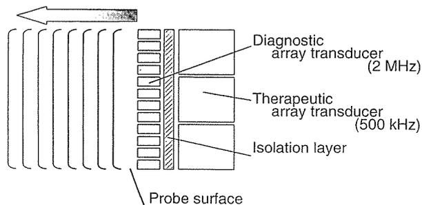
Fig. 2. Structure of T/D compound probe.
