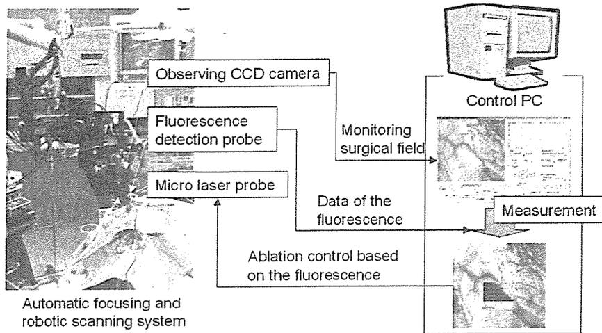
Fig. 4. System configuration
