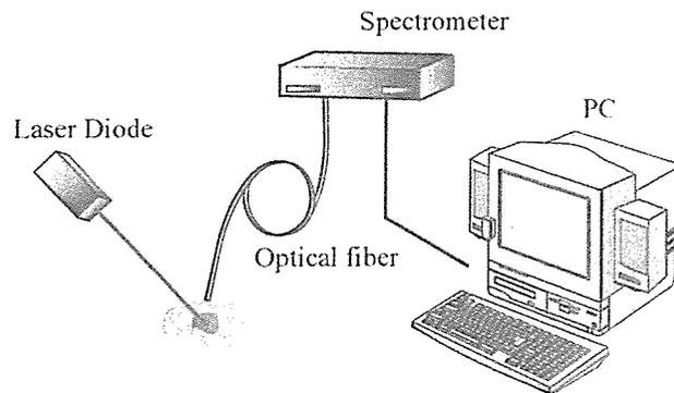
Fig. 1. Tumor detection system using 5-ALA-induced PpIX fluorescence
