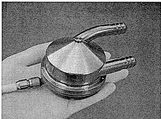
Figure 1. NEDO PI centrifugal pump (height of the housing: 37 mm, diameter: 55 mm).
