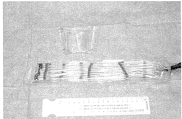
Fig. 2 Whole view of the mechanical artificial myocardium developed; the ventricle was covered by the band-shaped device and it was able to support the contractile function synchronising with natural heart beat.
