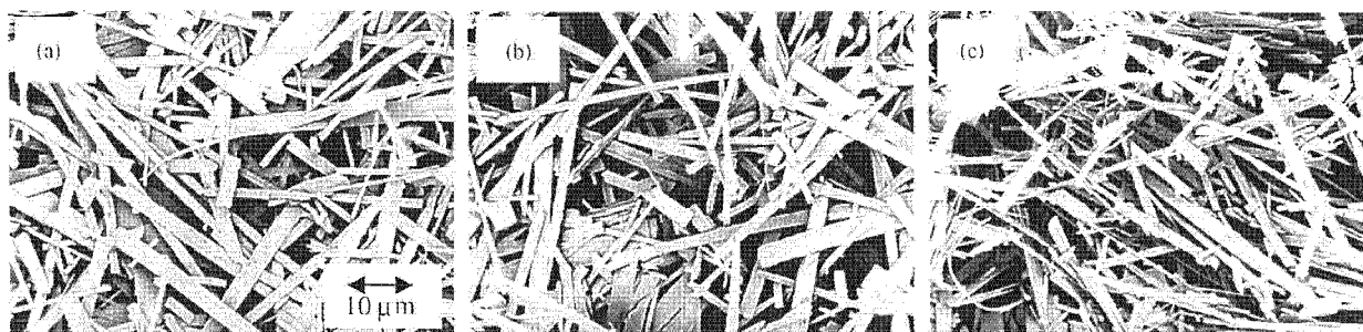
Fig. 6. SEM micrographs of the Ca-def HAp fibres synthesized from starting solutions with the Ca/P ratios of 1.00 (a), 1.40 (b) and 1.67 (c).
