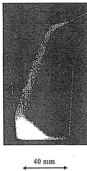
Figure 9: Radiogram of aluminum grains from a glass test tube.
