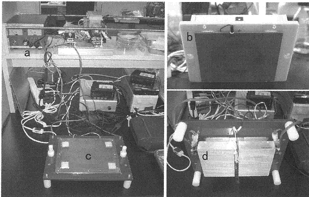
Fig. 1. Temperature-controlled semidry blotting apparatus.
