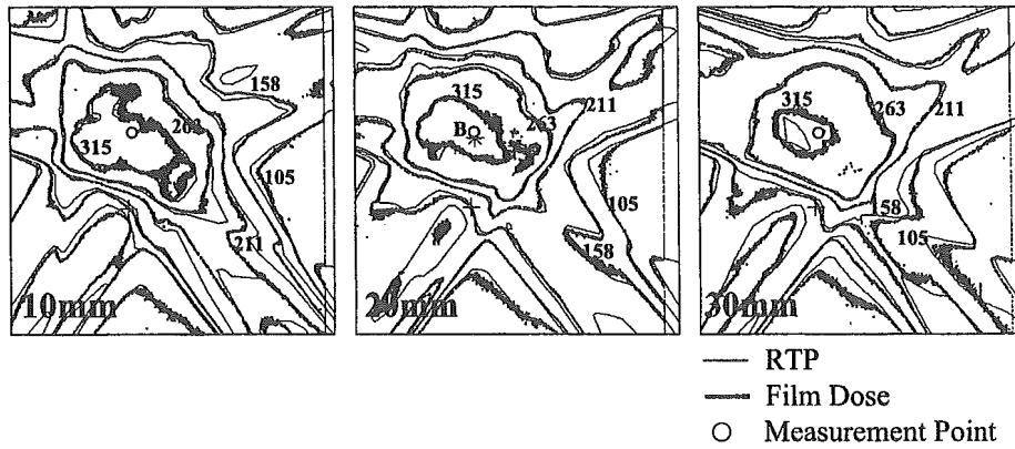
Fig. 5 Dose distributions of axial planes were derived from RTP and radiographic film at point B. The circle represents the points of measurement. The dose levels shown are in units of absolute dose.
