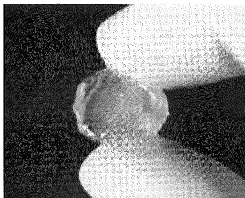
Fig. 2. Appearance of PLA-DX-PEG (reprinted from [51], with permission from Marcel Dekker Inc.) requires copyright permission since we previously published in Tissue engineering and novel delivery systems [51]. At room temperature, PLA-DX-PEG with a molecular weight of 9500 is a firm gel, which can be shaped and is easy to manipulate.
