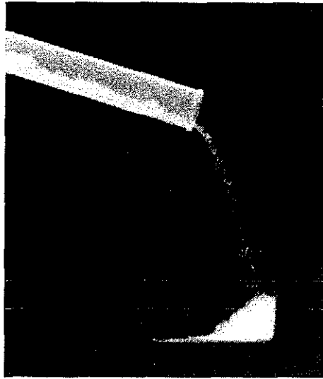
Figure 12: Radiogram of aluminum grains falling into polypropylene beaker from glass test tube.
