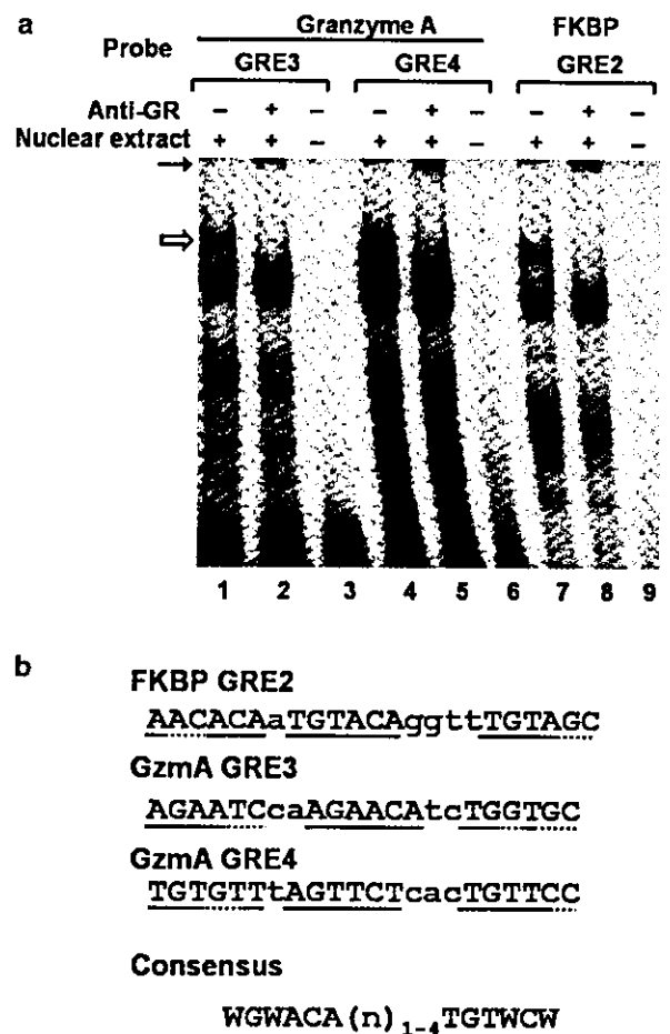
Figure 5 Electrophoretic mobility shift assays and alignment of GC-reactive sequences. (a) GR can bind in vitro to an oligonucleotide probe representing the GZMA and FKBP5 gene region. Nuclear extracts were obtained from COS-7 cells transiently transfected with expression plasmid for GR and incubated with 32 P-labeled oligonucleotide DNA probes containing putative GRE sequences with or without polyclonal antibody against GR as indicated. DNA-protein complexes were size-fractionated in a nondenaturing polyacrylamide gel and detected by autoradiography. The shifted and supershifted complexes are indicated by open and closed arrows, respectively. (b) DNA sequences demonstrated to be reactive to GC are aligned. The consensus motif deduced from the alignment is indicated at the bottom. Nucleotides that fit and do not fit into the consensus motif are indicated by solid and broken underlines, respectively. Lowercase letters indicate nucleotides that separate 5-bp consensus sequences. W indicates the nucleotide A or T.
