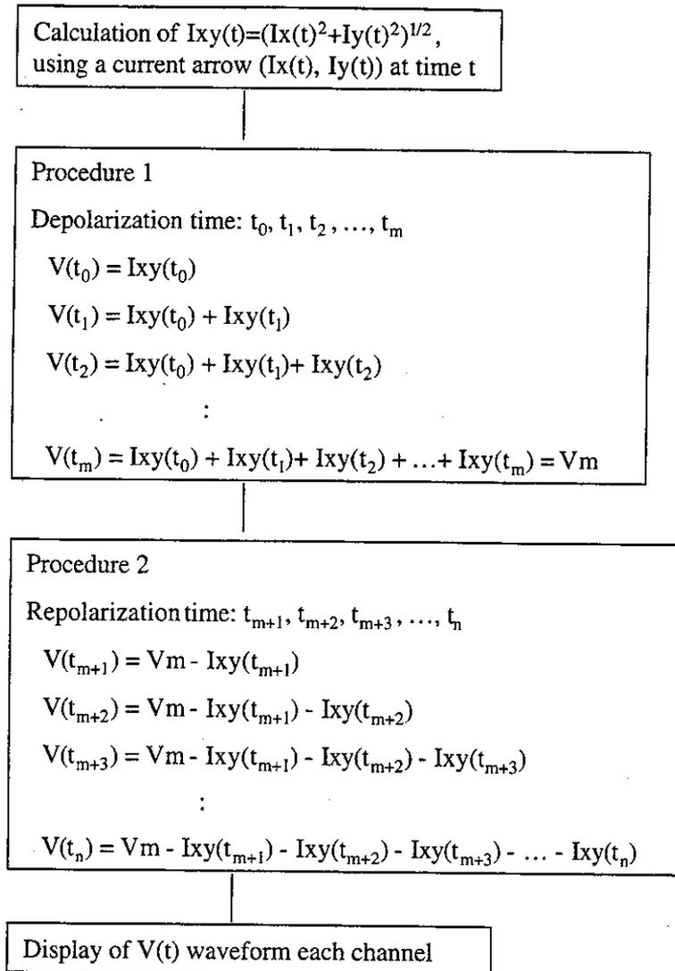
**Figure 4.** Flow chart for reconstructing an action potential.
