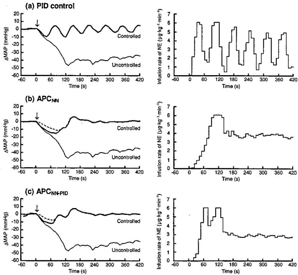
FIGURE 9. Typical examples of (a) PID control, (b) APC<sub>NN</sub>, and (c) APC<sub>NN</sub>-PID obtained from one animal in Protocol 1. The left panels show the MAP responses (thick solid line) and the uncontrolled condition (thin solid line). Dotted lines in (b) and (c) represent MAP responses predicted by the NN. Arrows indicate the start point of hemorrhage and MAP control. The right panels show the NE infusion rate.
