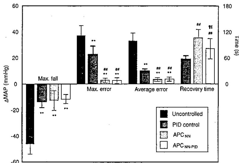
FIGURE 12. Maximum fall, maximum error, average error, and recovery time in the uncontrolled condition, PID control, APC<sub>NN</sub>, and APC<sub>NN-PID</sub> obtained from Protocol 2. \*\* $P < 0.01$  vs. the uncontrolled condition. ## $P < 0.01$  vs. PID control. ¶ $P < 0.01$  vs. APC<sub>NN</sub>.
