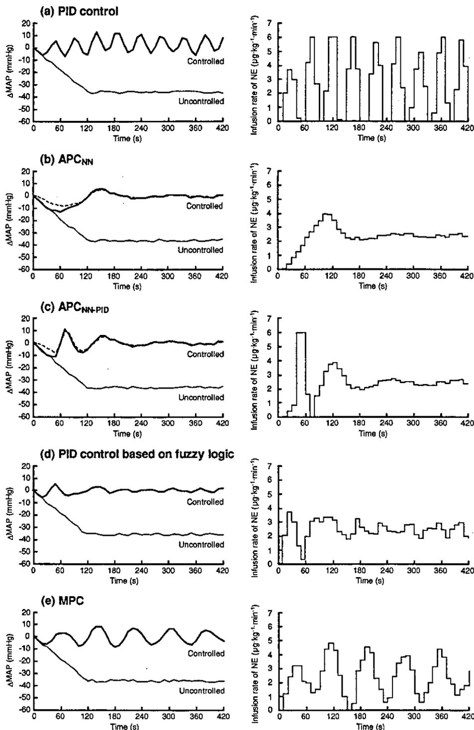
FIGURE 8. The simulation results of (a) PID control, (b)  $APC_{NN}$ , (c)  $APC_{NN-PID}$ , (d) PID control based on fuzzy inference, and (e) MPC under the unexpected MAP change. Left panels are changes in MAP and right panels are the NE infusion rate. Dotted lines in (b) and (c) represent MAP responses predicted by the NN.
