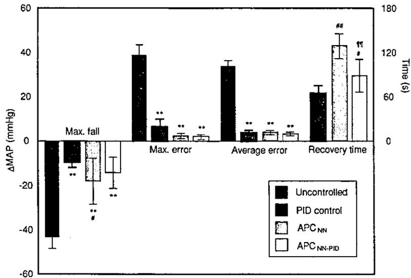
FIGURE 10. Maximum fall, maximum error, average absolute value of error between the target and observed MAP value (average error), and recovery time in the uncontrolled condition, PID control, APC<sub>NN</sub>, and APC<sub>NN</sub>-PID obtained from Protocol 1. \*\* $P < 0.01$  vs. the uncontrolled condition. ## $P < 0.01$  vs. PID control. # $P < 0.05$  vs. PID control. ¶¶ $P < 0.01$  vs. APC<sub>NN</sub>.
