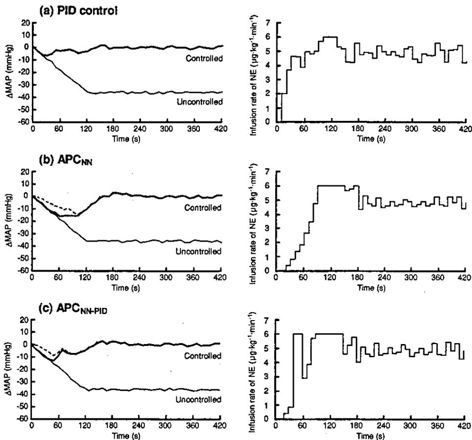
FIGURE 6. Simulation results of (a) PID control, (b)  $APC_{NN}$ , and (c)  $APC_{NN-PID}$ . The left panels show the MAP responses (thick solid line) and the uncontrolled condition (thin solid line). Dotted lines in (b) and (c) represent MAP responses predicted by the NN. The right panels show the NE infusion rate. Acute hypotension of  $-36$  mmHg was completed in 2 min and maintained thereafter.
