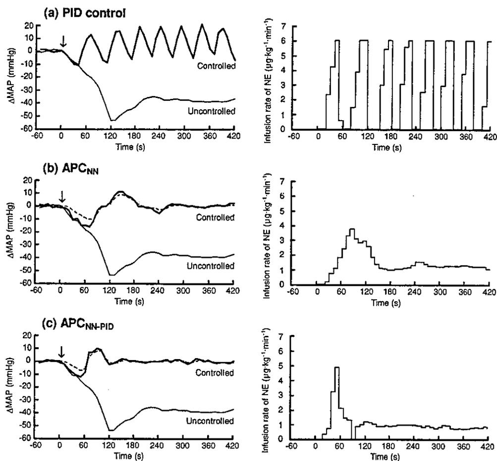
**FIGURE 11.** Typical examples of (a) PID control, (b)  $APC_{NN}$ , and (c)  $APC_{NN-PID}$  obtained from one animal in Protocol 2. The left panels show the MAP responses (thick solid line) and the uncontrolled condition (thin solid line). Dotted lines in (b) and (c) represent MAP responses predicted by the NN. Arrows indicate the start point of hemorrhage and MAP control. The right panels show the NE infusion rate.
