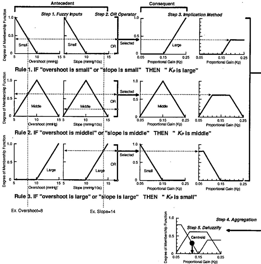
FIGURE 5. An example of a fuzzy inference system. The process for fuzzy inference is shown as Steps 1 to 5. The proportional gain ( $K_p$ ) in the improved PID control was updated through the process for the fuzzy Inference.
