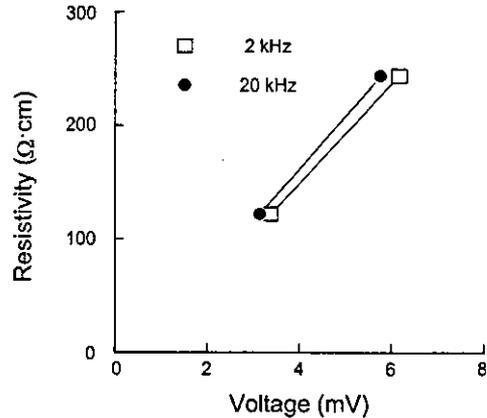
Fig. 9. Relation between measured voltage and saline resistivity.
