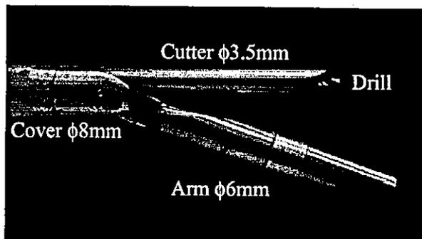
Fig. 5. End effector of the manipulator has the arm, cutter and drill. The end effector has 4 degree-of-freedom; 1) bending the arm, 2) translating the cutter, 3) rotating the drill and 4) rotating the end effector.
