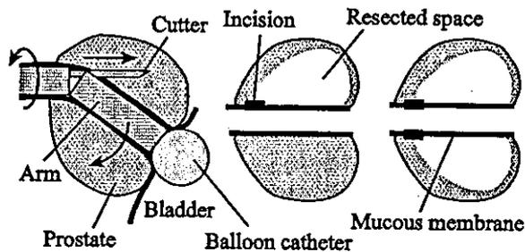
Fig. 2. Prostate displacement mechanism for minimizing damage to the mucous membrane. The end effector of the manipulator has the arm and cutter. Combination of the arm and cutter enable the manipulator to resect sufficient volume of the prostate tissue through small incision.
