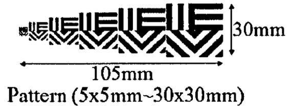
Fig.5 Resolution measurement chart.
