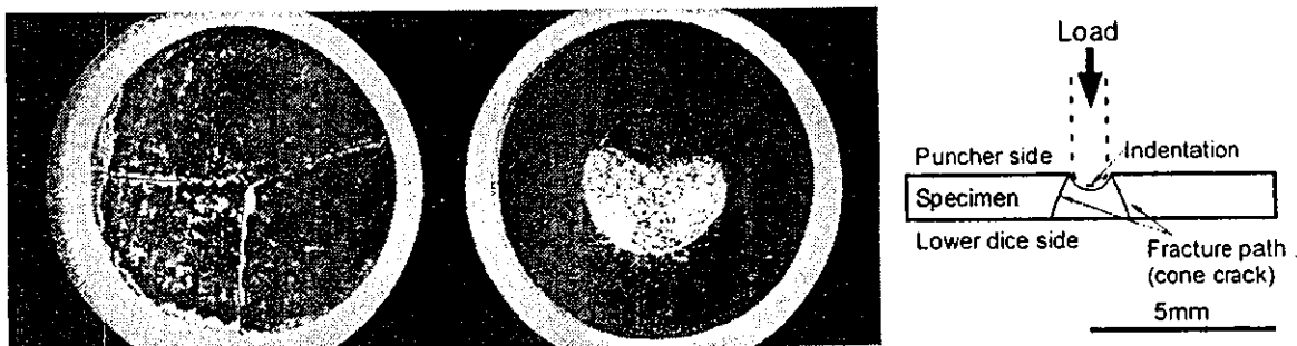
Fig. 7 Crack propagation of the unpurified SWCNTs (left) and Purified SWCNTs (center). Schematic illustration of the fracture path in the purified SWCNTs is also shown (right).
