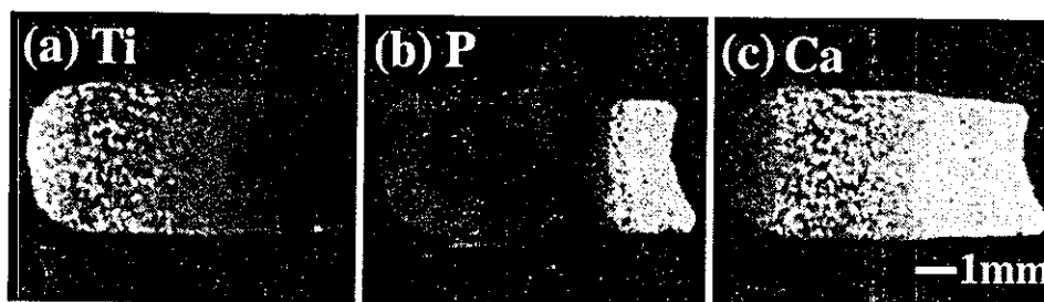
Fig. 3. XSAM elemental mapping of Ti/HAP FGM formed by sedimentation method. a:Ti, b:P, c:Ca.
