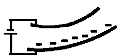
Fig. 4 Bending of the ion exchange polymer membrane caused by the shift of hydrated free anions
