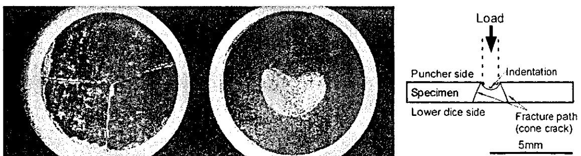
Fig. 7 Crack propagation of the unpurified SWCNTs (left) and Purified SWCNTs (center). Schematic illustration of the fracture path in the purified SWCNTs in also shown (right).
