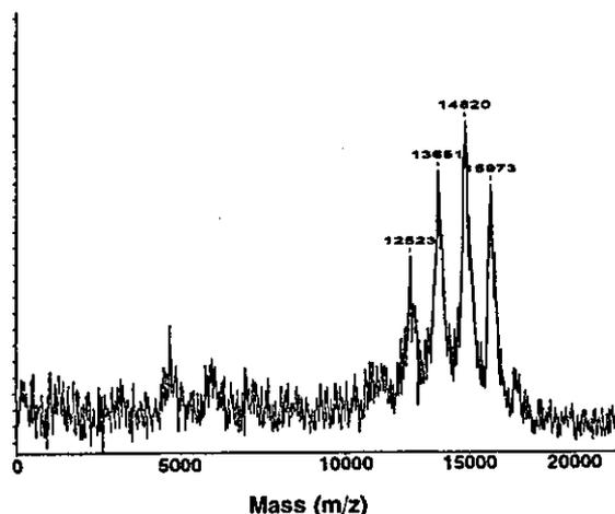
Fig. 2. MALDI-TOF-MS spectrum of carboasilane dendrimers carrying 12, 11, 10, and 9  $\beta$ -CD moieties.
