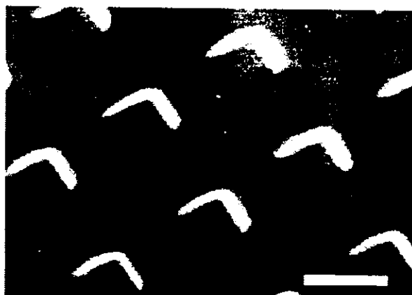
Figure 3. SEM of three-dimensional PDMS microstructures. Scale bar: 100 \mu\text{m} .
